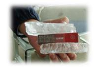
overheating refrigerants gas begin a heat exchange with the plate ice at the same time. The plate ice then loses adhesive force and the ice drops into the ice crushing gadget due to gravity. After the ice is off
