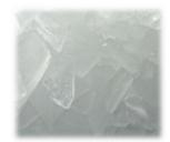
Plate ice introduction: Plate ice is a kind of irregular sheet ice with about  $40\times40$ mm $\sim80\times80$ mm in size, and 10 mm $\sim15$ mm in thickness. The thickness can be adjusted according to ice-making time with the maximum gauge being 25mm. Plate ice is a kind of thick and transparent ice which has good air permeability and a long shelf life.
